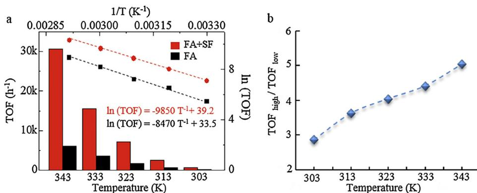
**Fig. 3.** Temperature dependence of FA dehydrogenation. (a) Arrhenius plot and TOF values of FA decomposition at different temperatures. Black line condition: FA 4 mol/L. Red line condition: [FA]+[SF]=6 mol/L, [SF]/[FA]=0.5. (b) TOF ratio under different conditions at same temperature in a.
