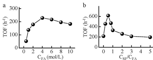
**Fig. 2.** Effect of FA concentration and the proportion of sodium formate (SF) to FA on the catalytic activity of IrCp\*Cl<sub>2</sub>bpy<sub>m</sub> for FA dehydrogenation. (a) FA concentration dependence of FA dehydrogenation at 30 °C. (b) Proportion of SF to FA dependence of FA dehydrogenation at 30 °C, [FA] + [SF] = 6 mol/L.
