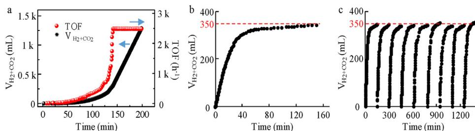
**Fig. 1.** Gas generation from FA dehydrogenation. (a) Gas generation process from FA dehydrogenation in the FA-SF mixture solution at 40 °C. (b) Gas generation from 300 μL FA in 4 mL water at 50 °C. (c) Cycles test of the FA dehydrogenation at 50 °C. Condition: catalyst (4.7 mg).
