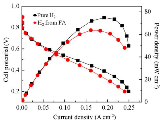
**Fig. 5.** Current generation by H<sub>2</sub> from FA dehydrogenation. Polarization curves of 2 cm<sup>2</sup> membrane electrode assembly (MEA) with different fuels. Anode and cathode: Pt loading (0.5 mg/cm<sup>2</sup>), gas rate from FA dehydrogenation (30 mL/min), pure hydrogen rate 15 mL/min.
